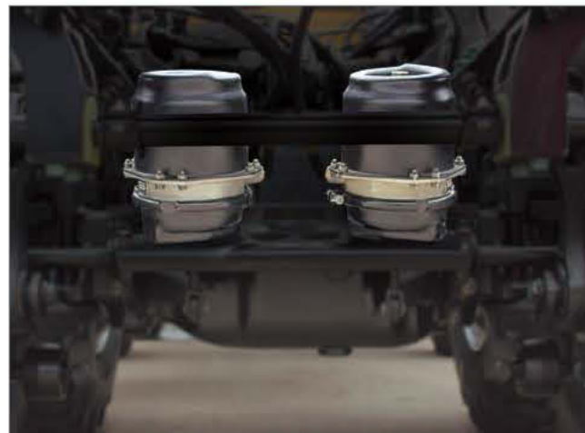
Elevated brake chambers
