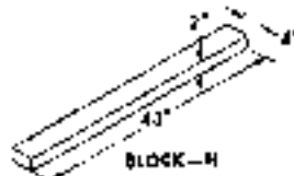
Figure 110 — Blocking Requirements for Securing Wheeled Vehicles on Railroad Cars
