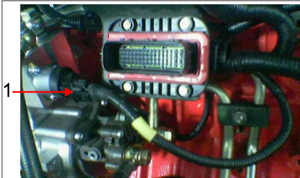
1. Fuel Metering Unit (MeUn) Connection on FIP
