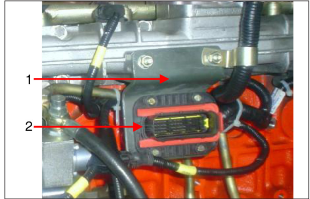
1. Bracket intermediate connector 2. Wiring Harness intermediate connector
