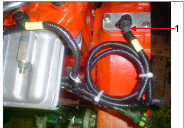
1. Crankshaft Speed Sensor Harness
