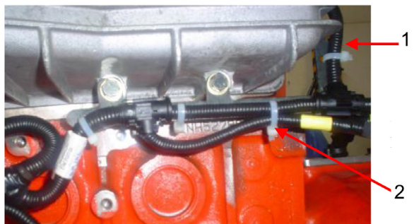
1. Rail Pressure Sensor Cable 2. Grid heater cable tied with bracket
