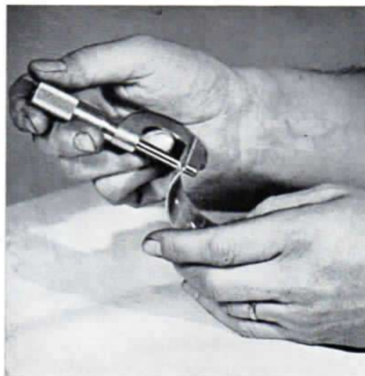
FIG. 26 CHECKING CONNECTING ROD BEARINGS WITH BALL MICROMETERS
