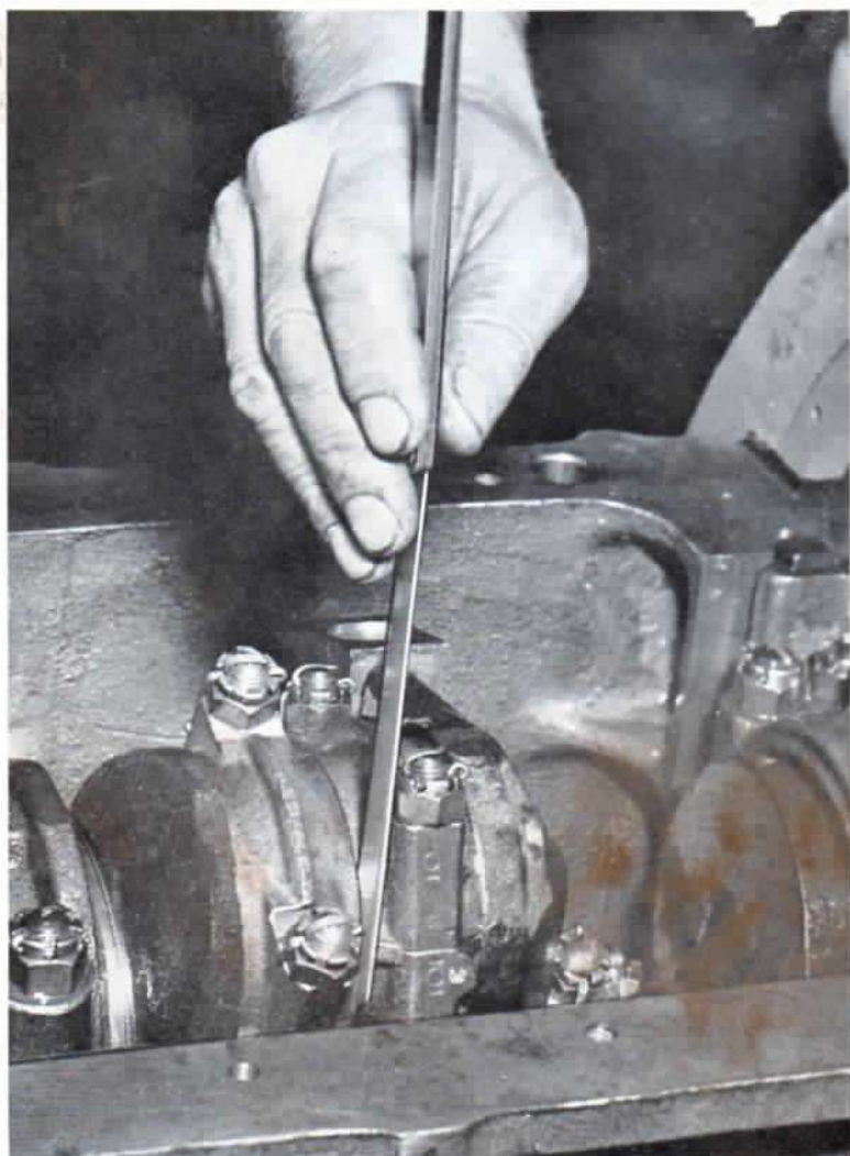
FIG. 29 CHECKING CONNECTING ROD SIDE CLEARANCE
